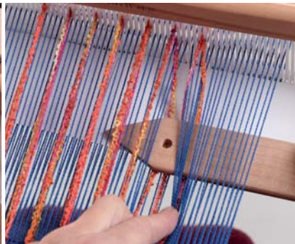
Deflect one supplementary warp from the right-hand pair and one from the left-hand pair and place under the stick
