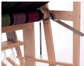
Easy action warp advancement with steel ratchet
