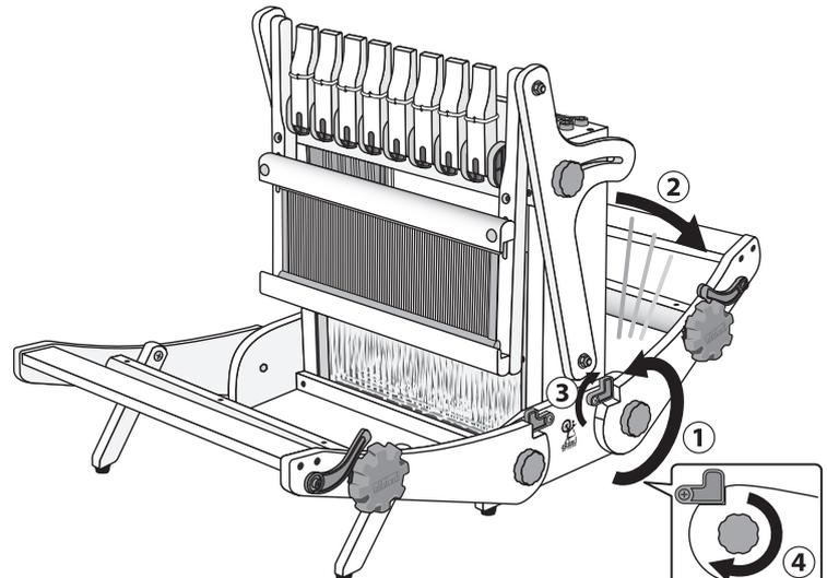
**Step 4:** Loosen knobs securing the beater supports, slide the beater completely forward and tighten the knobs.
