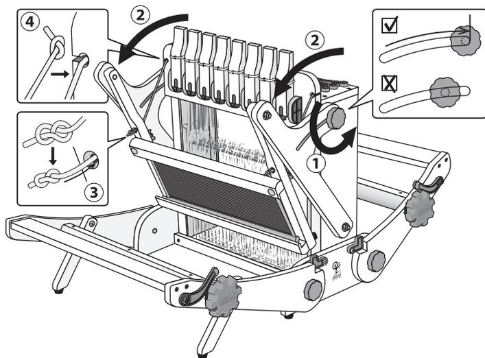
**Step 6:** Push the levers down and check the gap between the shafts and the castle top is approx. 1cm (1/2ins) on both sides. Adjust the height as necessary by moving the Texsolv cord in the lever or on the screw head in the shaft end.
