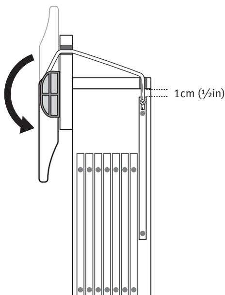
**Step 7:** Attach the front and back warp sticks with the cotton string supplied with your loom as illustrated.
