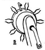
Place the wheel in position between the legs and insert the crankshaft. This has deliberately been made a tight fit in the hub so do not lubricate or ream out the hole. To secure the wheel first locate the hole in the crankshaft by pushing a fine knitting needle or nail through the lead hole in the hub. Hole in crankshaft is in line with crank. Twist the crankshaft backwards and
