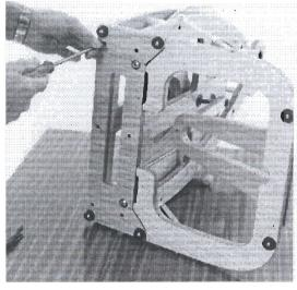
4 Use a hammer and tension pin to tap the flyer shaft and crank forward until they are free of the bearings in the back frame.
