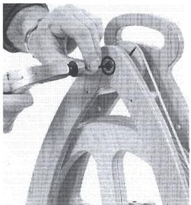
5 Lift the back frame away from the front flyer shaft and crank.
