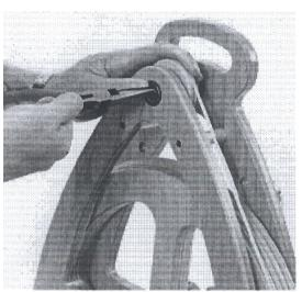
2 Remove the four screws that retain the back frame to the four dowel spacers.
