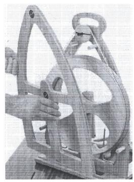
Carefully remove the E-clip from the front of the flyer shaft and slide the shaft out. Carefully remove the E Clip from in front of the pulley and slide the pulley off the shaft. Tap the new tension pin through the hole in the new flyer shaft. Slide the pulley onto the new flyer shaft until the groove engages the tension pin. Then secure with an E Clip. Fit the new shaft into the frame and secure with an E Clip.
