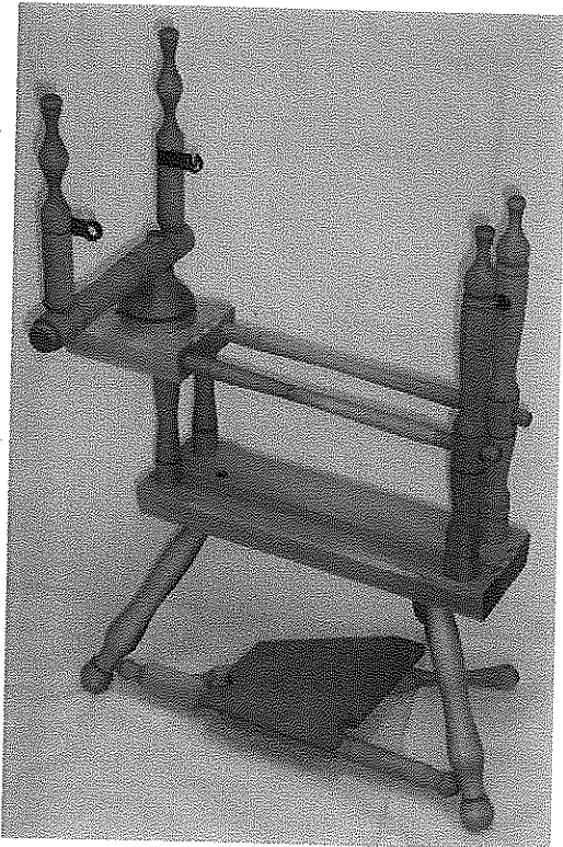
7) Thread the adjusting rails into the wheel supports. Then position the wheel & maiden bar supports into the base. Twist the rails to align the wheel with flyer and bobbin whorls.
