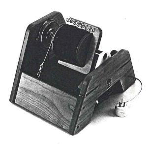
PS A nylon bush that may be inserted into the flyer orifice to reduce the diameter is included in the kit. This is beneficial when spinning finer yarns as it will help prevent the yarn vibrating. By spinning the yarn at about a 45 degree angle to the orifice the vibration will almost be eliminated. When plying or spinning thick yarns, remove the bush.
