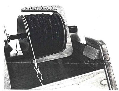
Step 6: Fold the front flyer bearing up and locate the flyer orifice into the bearing at the same time.
