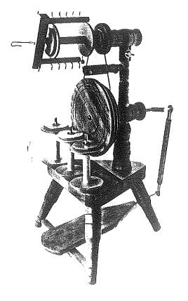
If there is too much tension on the brake band, the yarn will pull in too quickly or break.
