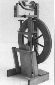
(16) Fit the tension knob into the top rail H. Knot the nylon at one end and thread through the tension knob, under the hook, over the bobbin end and tie to the tension spring. Place spring on the hook on the opposite side.
