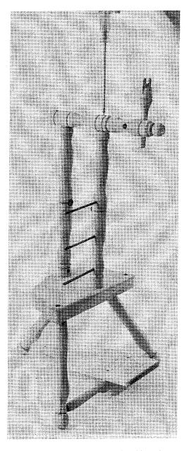
12) Locate the crank into the wheel bearings.
