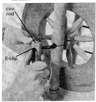
18) Locate the flexible conrod joint into the hole in the treadle board and secure with a 5/8" (16 mm) round head screw. Note: the treadle board should be parallel with the floor when the crank is to the bottom.
