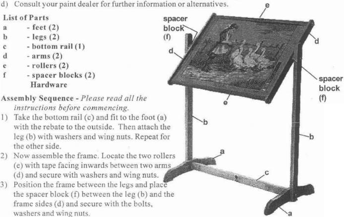
Your Ashford Tapestry Frame is now ready to use. Sew your tapestry to the tapes on the rollers, keeping the edges of the tapestry parallel on the frame. Adjust the tapestry to a convenient working height and angle using the slots and holes in the arms. Tighten the wingnuts to prevent the rollers turning and to keep the tapestry taut.
