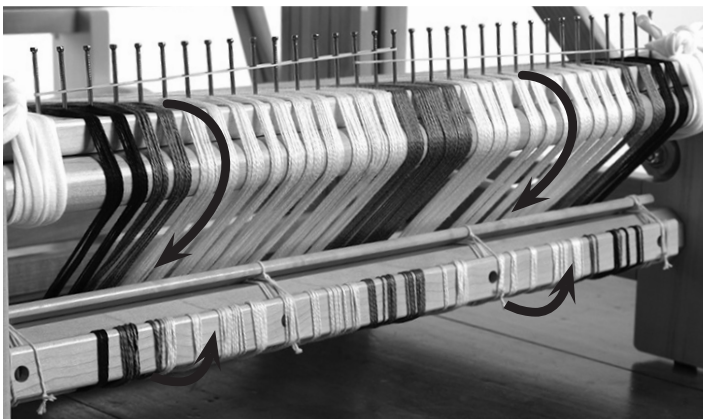
Winding the warp on the back roller.
