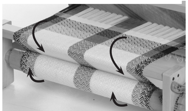
Winding the warp on the front roller.
