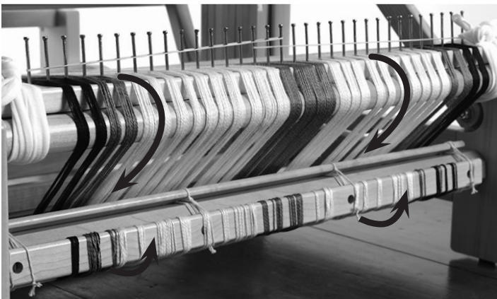
Winding the warp on the back roller.
