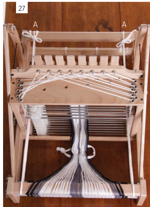
Attach 'helping hands' (stretchy cord included in the raddle kit) to the loom. On each side go from the front beam, through the castle, around the back beam, back through the castle and tie at the front beam (see A).
