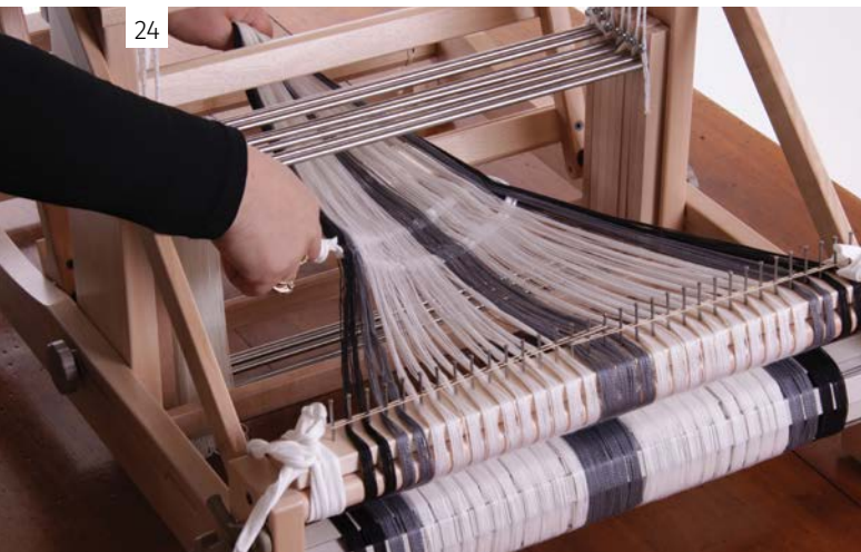
Wind on until the threading cross arrives behind the castle.
