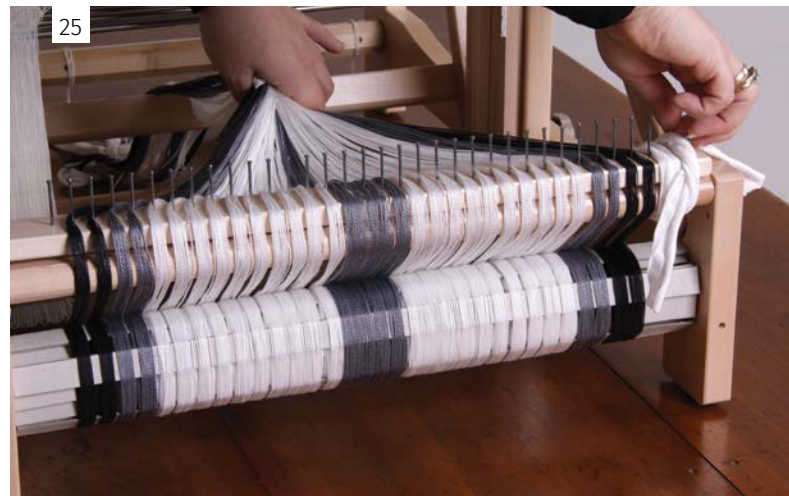
To remove the raddle, hold the warp up slightly, remove the rubber bands and the ties.
