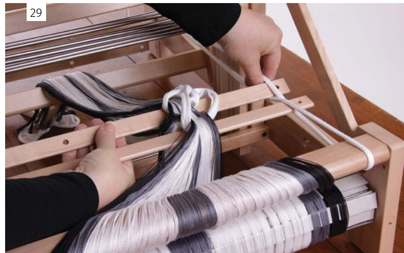
To support the cross sticks, use the helping hands, crossed in a figure eight.
