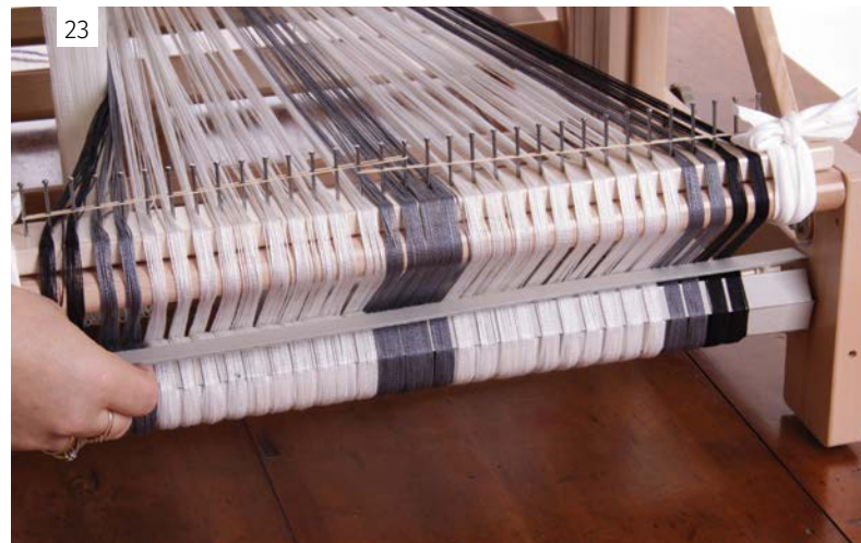
Continue beaming, inserting a cardboard warp stick at each revolution of the roller to separate the warp layers and allow the warp to beam even and smoothly.
