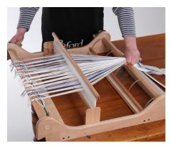
16. Untie the warp from the front roller. Now it's time to wind the yarn onto the back roller, keep the warp under tension. A friend can help by holding the end of the chain out under tension at the front of the loom.
