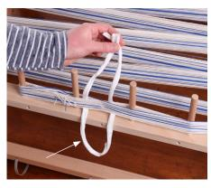
6. When all the yarn has been wound on, add choke ties to the warp to prevent tangling. Add a long loose tie through each side of the threading cross. NOTE: For wide projects wind your warp in two or three separate chains.
