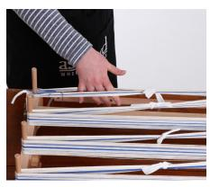
8. Now it is time to chain the warp from the pegs. To remove the warp begin at the end peg. Take your hand through the middle of the loop.
