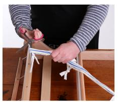
12. Holding the chain near the threading cross cut the top loops.
