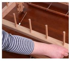
Tie the warp yarn to the start peg with a loop. Wind around the pegs for the required warp length and return following the same path back to the beginning.
