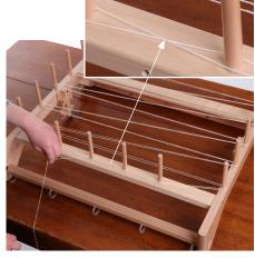
3. When returning back to the start you will be creating a threading cross between the second to last peg spacing. Create this cross by passing the thread up or down in the opposite direction to the previous thread. The threading cross keeps the yarn in the correct order for threading.
