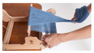
5. Insert a cardboard warp stick or piece of paper the full width of the loom. Continue adding cardboard warp sticks (1 in each rotation) or paper as you wind the warp on.
