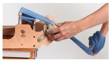
4. Stand at the back of the loom. Turn the back handle towards you allowing the threads to pass through your hand. Wind until the back warp stick goes around the roller once.
