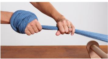
2. Twist the threads around your hand, maintaining an even firm tension, until you reach the front roller.
