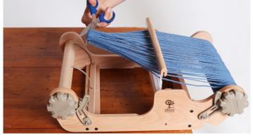
6. Stop winding once the yarn loops reach the front of the loom. Cut through the yarn loops. Unclamp the loom and follow the 'Learn to weave' booklet for threading the reed.
