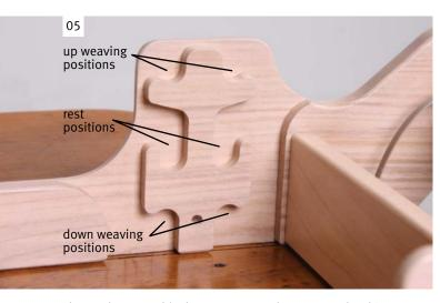
The reed support block can accommodate two reeds. This project only uses one reed.
