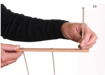
Connect the front and back warp sticks to the rollers with the warp stick ties. Push the arrowhead of the nylon ties through the holes in the warp sticks.
