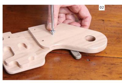
On the right loom side (with the brand) remove the protective wooden packer from the metal clicker pins, put the pawl in place, turn the loom side over and attach both pawls with a 20mm (3/4in) round head screw. NOTE the "clicker pin" fits into the gap of the pawl. Rub a little candle wax on the thread to make assembly easier. DO NOT over tighten. The pawls should move freely. **Leave 0.5mm** (1/32in) gap under the head of the screws.
