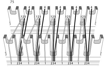
Continue across the reed. *Note: Check there are no crosses between the reeds.* If the ends are crossed remove and repeat step 74. Your threading will look like this diagram. Tie to the front warp stick following steps 20 - 26.
