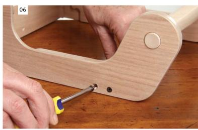
Locate both rollers into the left side and secure the front and back rails with wood screws.
