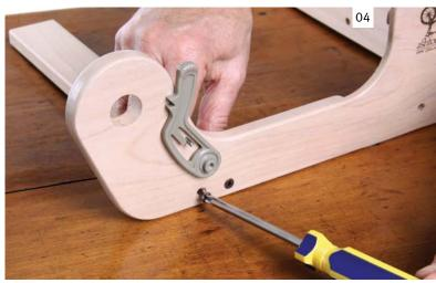
Secure the front rail to the right side with two wood screws. *Note:* Ensure the groove on the front rail is facing up.
