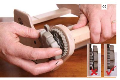
Locate the 4 pins on the handles into the 4 holes in the cogs. Then give the handle a sharp hit with the palm of your hand or a rubber hammer so they snap down tight onto the cogs.
