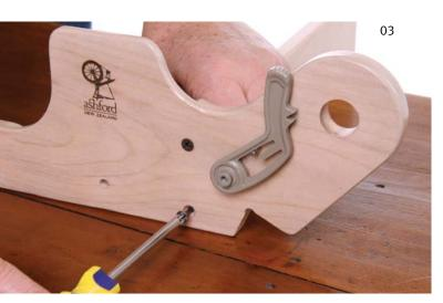
Secure the back rail to the right side with two wood screws. **Note:** The clamp hole is towards the bottom.
