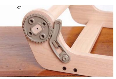
Place the cogs onto the ends of the rollers. Check the teeth engage the pawls.
