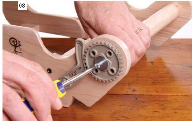
THEN secure with washers and 20mm (3/4in) screws.
