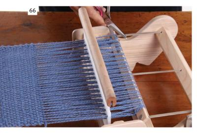
When you reach the end leave enough warp for your fringe. Cut the weft yarn and leave the end out. Cut the warp yarns along the back warp stick. Take care not to cut the warp stick ties.
