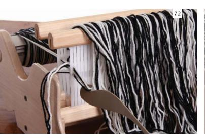
Place the second reed in the front rest position. Drape all ends from the back reed over the front reed (this will help to make the threading easier). Starting on the left, take the first group of 4 ends (2 white ends and 1 black end from the slot and 1 end from the eye to the right and thread all 4 ends through the slot directly in front in the front reed.
