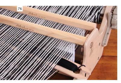
Plain weave - One layer double the ends per cm/in Place both reeds in up position, weave one row. Place both reeds in the down position, weave one row. Repeat step 1.
