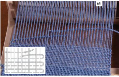
Joining in a new thread: At some stage the yarn on the shuttle will be finished. Wind some more yarn on the shuttle. Overlap the new yarn across the old yarn into the same shed. Beat both yarns together.
