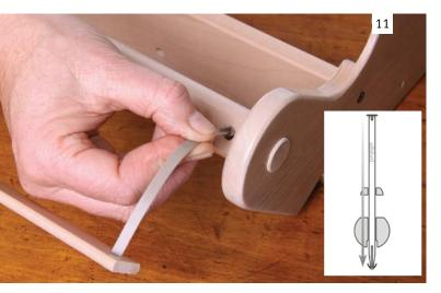
Then push the arrowhead ends into the small hole in the roller and out the larger hole as illustrated.
