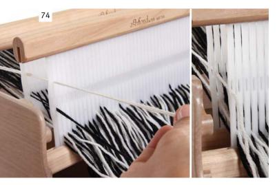
Take the first group of 4 ends and pull the black pair down and the white pair up. Take 1 white end from the pair of white ends and thread through the eye to the left.
