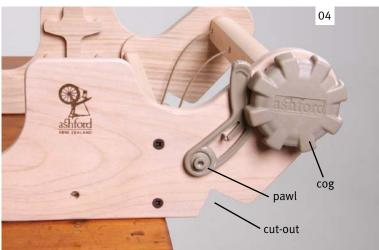
**Note:** The back of the loom has the cut-out in the lower edge. Engage the front and back pawls into the teeth in the cogs.
