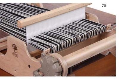
Place one reed in the back rest position. Warp across reed in the normal way but place two loops in each slot (one loop of black and one of white). Follow steps 12 - 19 to finish the warping sequence.
