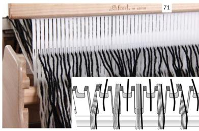
With the front of the loom facing you and starting from the left use a threading hook to take one of the black ends from the slot and thread it through the eye to the right. Continue across the reed.
