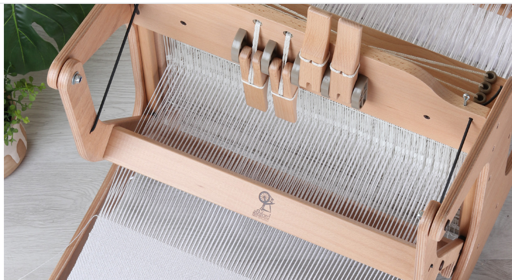
Split pins hold reed in place when sleying
