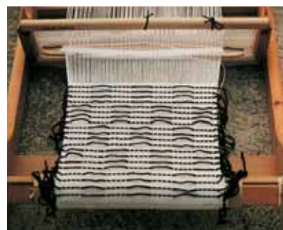
Rigid heddle loom with fabric and shibori wefts. The chosen shibori thread needs to be strong, non-stretchy and smooth so that it will pull the fabric into pleats and resist the dye type you've chosen
