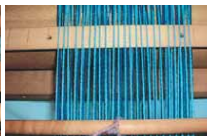
See how the hole threads for the back and front heddles are reversed
