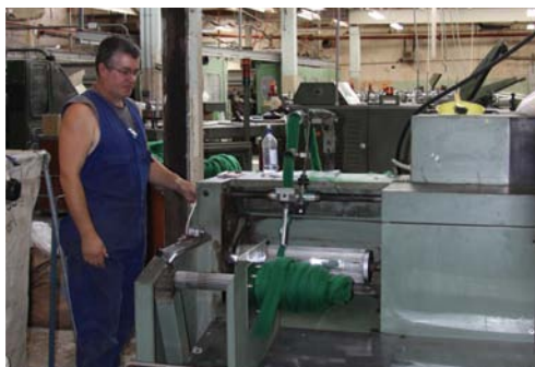
Wayne controls the baller which converts the wool into 1kg (2.2lbs) bumps
