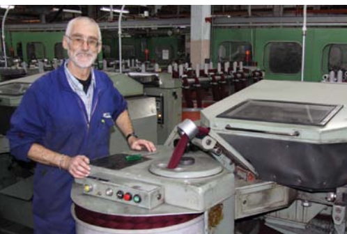
Louis adjusts the auto-leveler that produces a standard thickness or kilotex (grams per metre)
