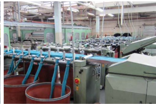
The wool is gilled and combed to remove any short pieces and to align the fibres
