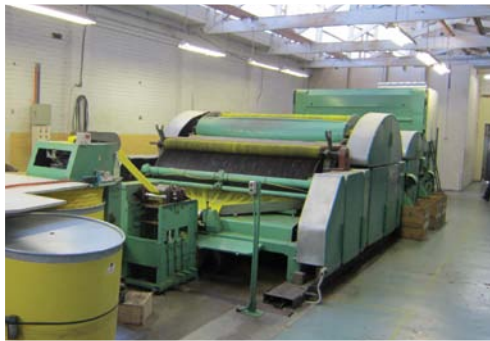
After the wool is dried it is carded and formed into a tape
