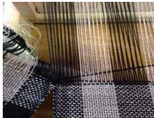
The warp from Piece A becomes the weft in Piece B
