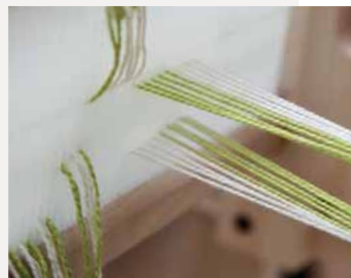
Thread the loom so when green is on top, natural is on the bottom (and vice versa)
