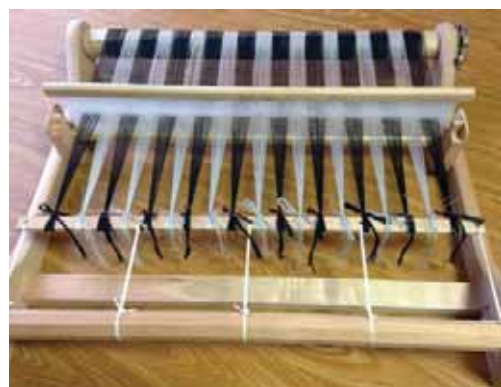
Warp the loom alternating with the black and the light-reflecting grey yarn
