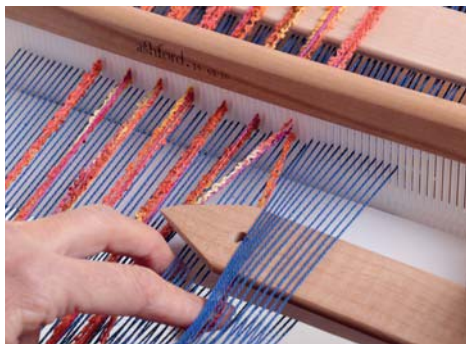
Bring pickup stick C to the surface two slot threads of the background warp before the supplementary warp threads and deflect one of the supplementary warp threads under the pickup stick C
