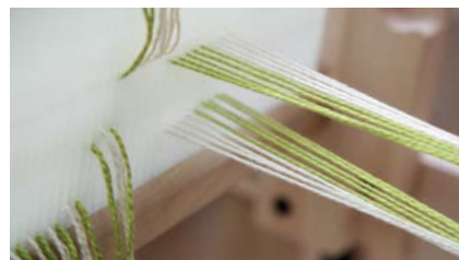
Thread the loom so when green is on top, natural is on the bottom (and vice versa)
