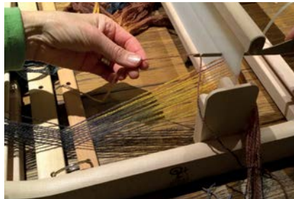
Thread from the front to the back through each eye and slot.
