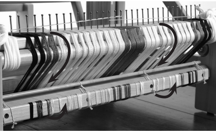
Winding the warp on the back roller.
