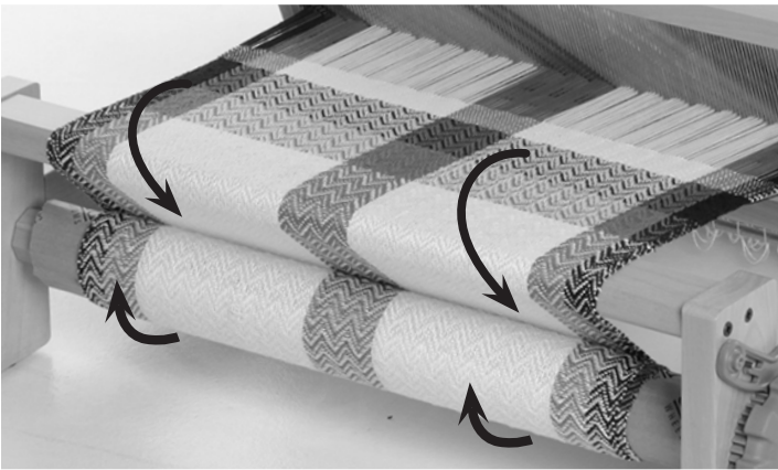
Winding the warp on the front roller.
