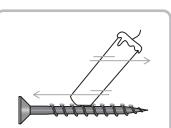
To make assembly easier use candle wax on the screws.
