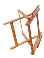
7. Lay the loom stand base on it's side and place the top of the stand in position - make sure the front of the shelves are at the opposite end of the spacer rails with the Ashford logo.
