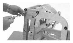
**4.** Use a hammer and nail to tap the flyer shaft and crank forward until they are free of the bearings in the back frame.
