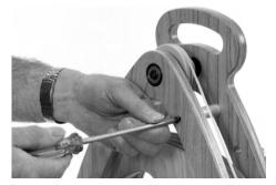
**3.** Remove the three screws that attach the back frame to the base.
