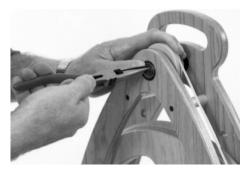
**2.** Remove the four screws that retain the back frame to the four dowel spacers.
