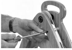
**3.** Remove the three screws that attach the back frame to the base.
