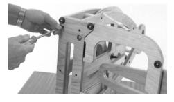
**4.** Use a hammer and nail to tap the flyer shaft and crank forward until they are free of the bearings in the back frame.
