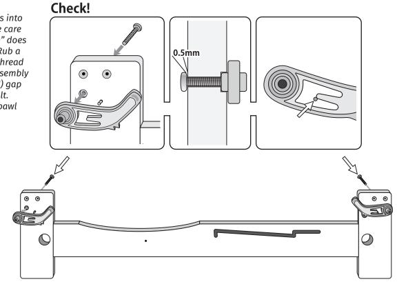
Rub candle wax on the dowel ends of the rollers. Place the rollers into the holes in the loom sides. Attach the front and back beams to the sides with 50mm (2") screws. Check the round edge of the beams face out.
