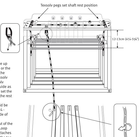
Move the levers into the up position on the 4 shaft or the 4 right hand levers on the 8 shaft loom. Insert Texsolv pegs through the Texsolv cord beside the cord guide as illustrated. These pegs set the height of the shafts in the rest position.
