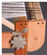
second back beam 2nd back roller and beam for perfect tension when warping with different yarns on your table loom.
