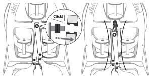
**Double treadle:** Before folding, click the outside conrod off, then rotate the wheel so the inside crank is to the bottom. This avoids unnecessary stress on the conrod, flexible joint or bearing.
