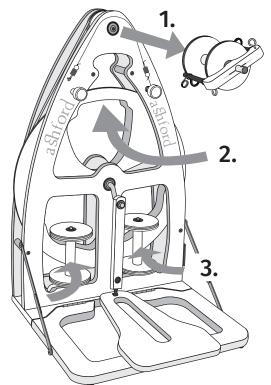
**Single treadle:** Before folding always rotate the wheel so the crank is to the bottom. This avoids unnecessary stress on the conrod, flexible joint or bearing.
