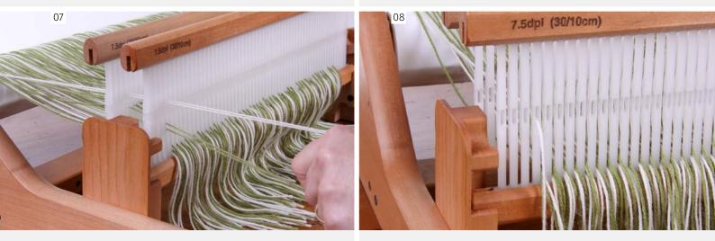
Place both reeds in the rest position. Take the first group of 4 ends and pull the moss pair down and the white pair up.
