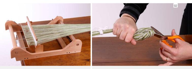
Place one reed in the back rest position. Excluding the first three and last three slots, warp across the reed in the normal way but place two loops in each slot, one loop of moss and one of white (4 threads in each slot).
