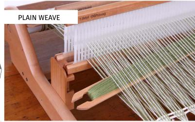
PLAIN WEAVE - One layer double the ends per cm/in. Place both reeds in up position, weave one row. Place both reeds in the down position, weave one row. Repeat these steps. *Hint:* When changing the shed leave the front reed hanging.
