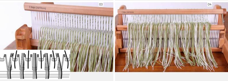
With the front of the loom facing you, starting from the left, use the threading hook, take one of the moss ends from the slot and thread it through the eye to the right. Continue across the reed. Place the second reed in the front heddle down position. Drape all ends from the back reed over the front reed (this will help to make the threading easier).
