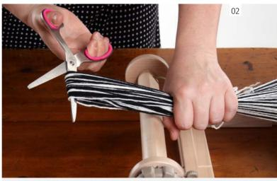
Wind the warp onto the back roller and cut the loops. (See steps 12 - 19 in the Learn to weave on the SampleIt Loom booklet for detailed warping instructions).
