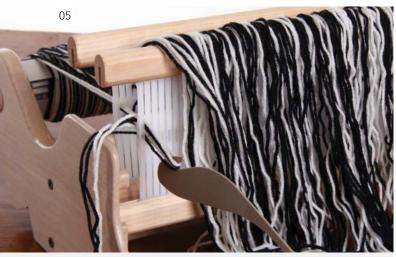
Starting on the left, take the first group of 4 ends (2 white ends and 1 black end from the slot and 1 end from the eye to the right) and thread all 4 ends through the slot directly in front in the front reed.
