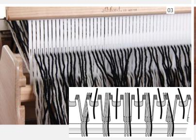
With the front of the loom facing you, starting from the left, use the threading hook, take one of the black ends from the slot and thread it through the eye to the right. Continue across the reed.
