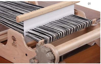
Place one reed in the back rest position. Warp across the reed in the normal way but place two loops in each slot, one loop of black and one of white (4 threads in each slot).
