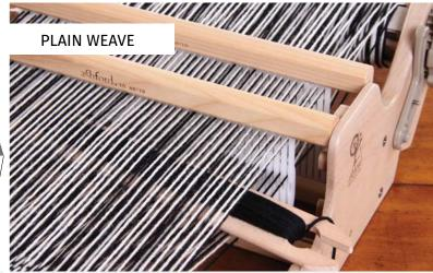
PLAIN WEAVE - One layer double the ends per cm/in. Place both reeds in up position, weave one row. Place both reeds in the down position, weave one row. Repeat these steps.
