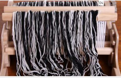
Place the second reed in the front rest position. Drape all ends from the back reed over the front reed (this will help to make the threading easier).
