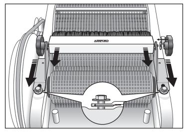
5. Rotate the packer brush until the bristles are about  $\frac{1}{2}$  way into the carder teeth, then tighten the 2 knobs.
