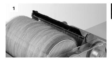
Load your carder with fibre as normal. When the drum is full remove the cover, lift the packer brush up and out of the teeth, turn the **switch to unwind** and turn the speed down so the drum rotates slowly. Rotate the drum until you see the metal strip.
