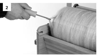
Using the awl (doffer) separate a small portion of the fibre at the edge of the drum.
