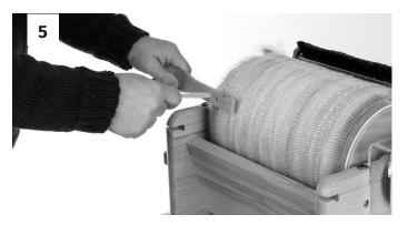
Pinch the fibre firmly and pull through the diz stick while the drum rotates. Do not pull too far as the fibre will separate.
