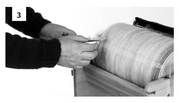
Fold the end of the fibre over and twist a little in your fingers to make it easier to thread through the hole from the countersunk side.
