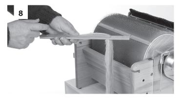
Once you have removed the entire batt, hold a length of fibre along the diz stick and wrap the sliver around the diz stick to form your bump.
